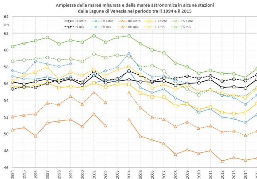
Fig. 5 – Variation in tidal amplitude using the extremes relative to a single astronomic component (continuous line) and the complete tidal signal including the meteorological contribution (dotted line) in some stations of Fig. 2.
