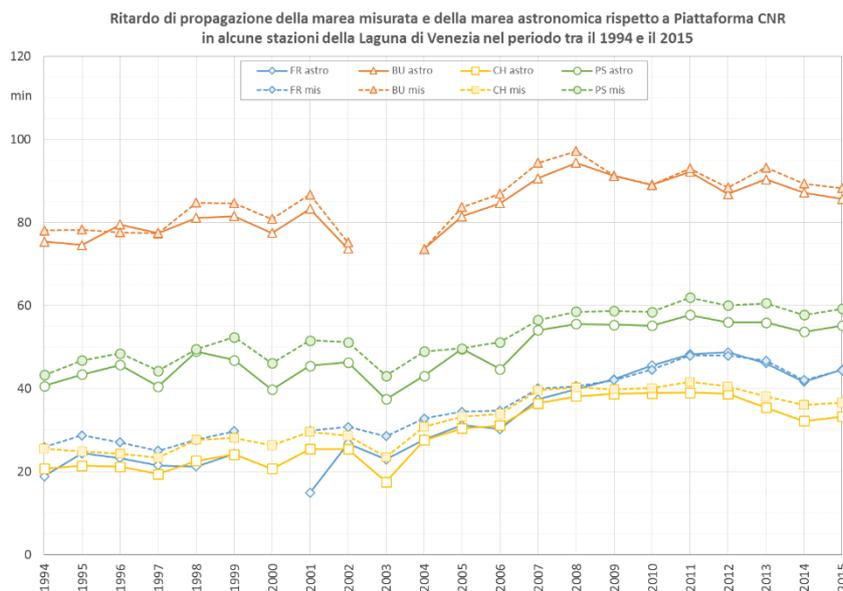
Fig. 6 – Variation in the tide propagation delay obtained by analysing the extremes relative to a single astronomic component (continuous line) and the complete tidal signal including the meteorological contribution (dotted line) in some of the 4 stations of Fig. 2.
