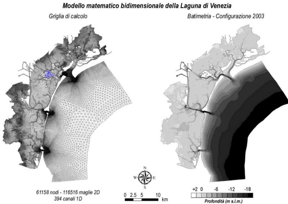
Fig. 7 –Calculation grid and bathymetric scheme of the bidimensional model of the Venice Lagoon.
